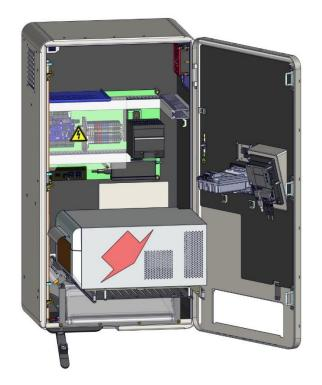
Pull out the printer forward until it stops.
